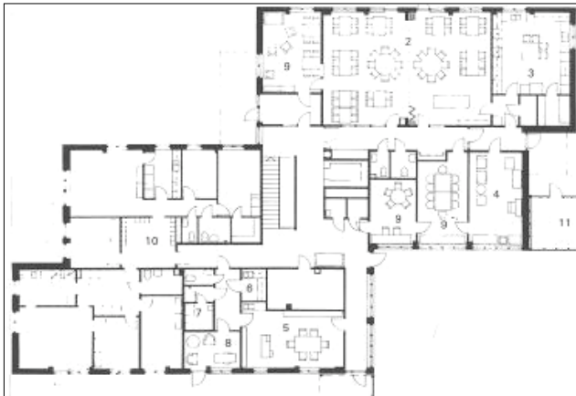
Figure 13. The ground floor of Prästgårdshagen. It was designed to stimulate spontaneous use of common spaces.
