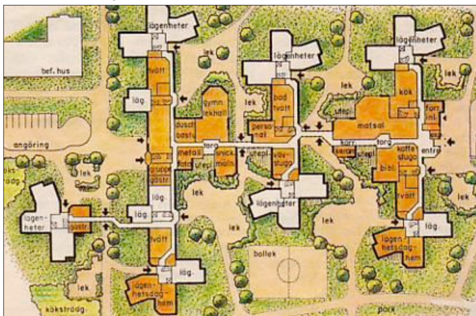
Figure 15. Ground plan of Stolplyckan in Linköping – 184 apartments, connected under cover and with a staffed reception, dining hall, cafeteria, library, club-rooms, two day care centres, exercise-rooms, weaving workshop, carpentry workshop and several laundries.
